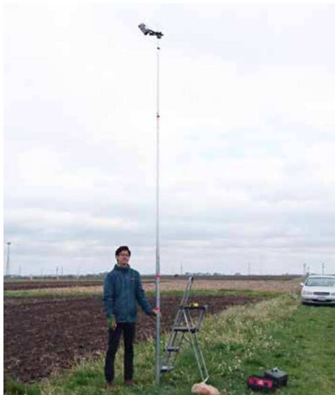
University of Illinois doctoral student Hyungsuk Kimm set up a network of cameras in corn fields around Illinois to ground-truth satellite-based algorithms to monitor corn productivity in real time. Photo credit: Hyungsuk Kimm, University of Illinois.
