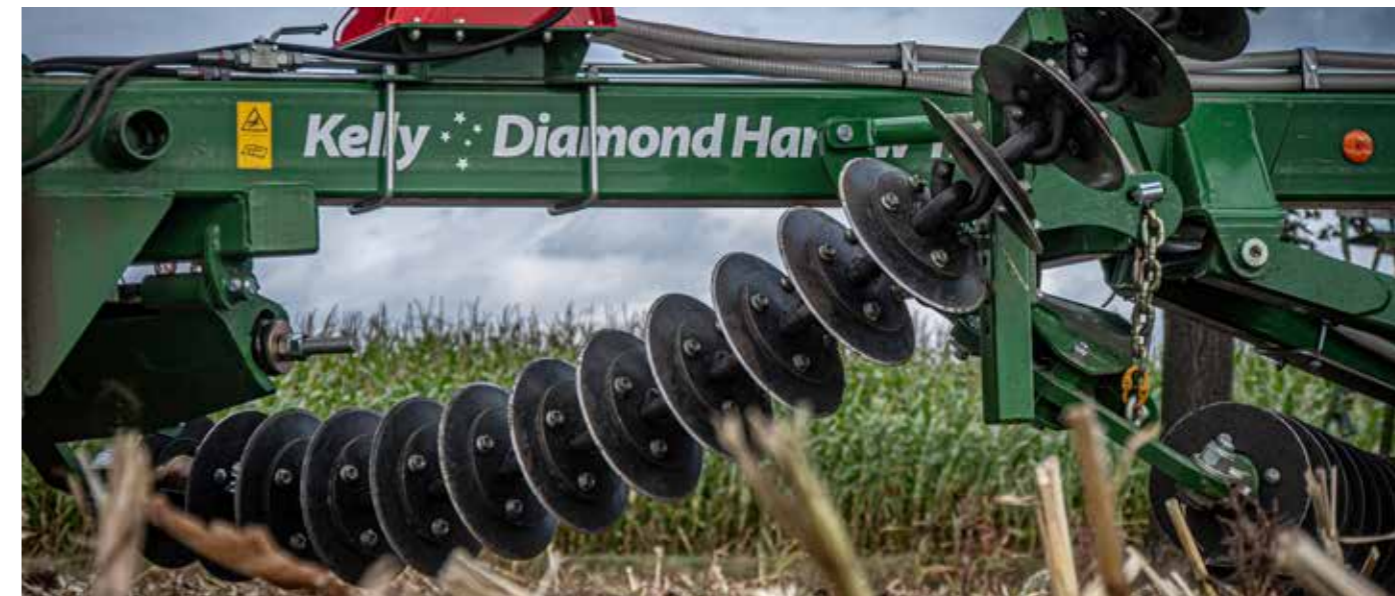
The blunt discs can be swapped for these sharp discs and used to kill the weed seedlings that germinate after one pass with the blunt discs on the chain.
