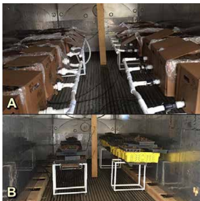
A, The precision thermotherapy unit setup for the high-elevation nursery trial in 2016. The extended setup allowed treatment of 18 boxes and employed four vacuums. B, The setup used for the trials at Escalon and Ballico in 2017. A similar setup was used for the grower-run trial in 2018.
