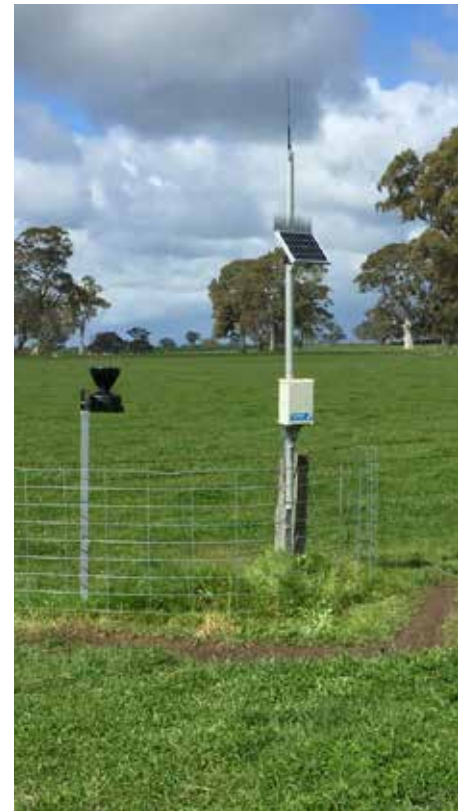
Soil moisture monitoring probe setup.
