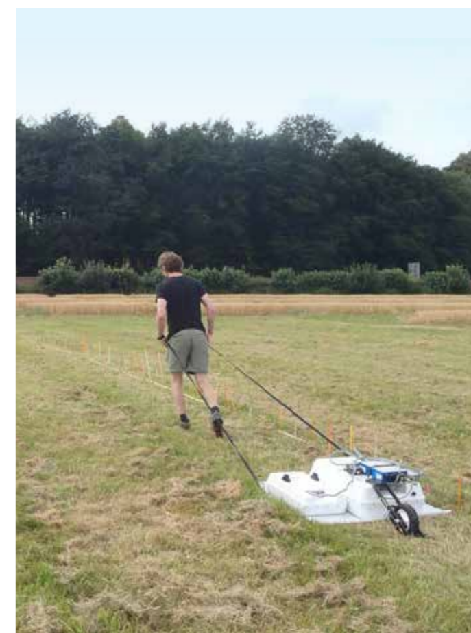
Lee Slater, dragging the ground penetrating radar equipment over the soil's surface. Credit: Chris Watts, Rothamsted Research.
