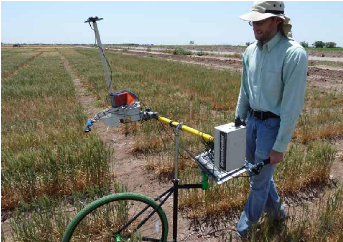
Kansas State University student and phenocart developer Jared Crain collects data using the phenocart in drought stress wheat trials at the Norman E. Borlaug Research Station, Cd. Obregon, Mexico.
