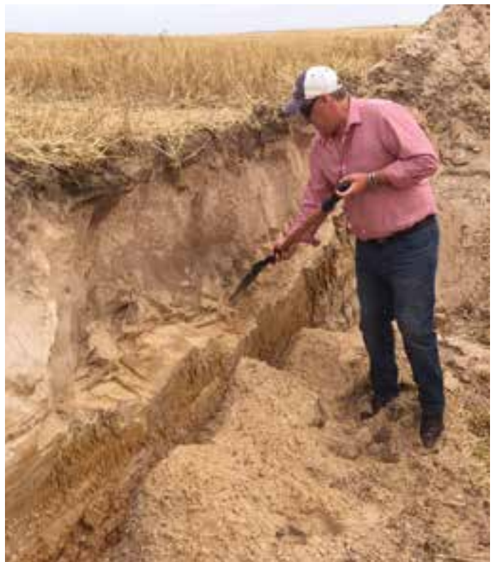
Soil Pit Profile - Deep Sand over Sodic Clay - Yorke Peninsula S.A.
