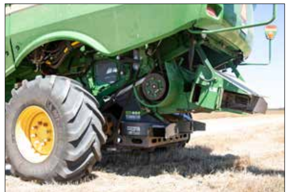
Impact mills provide the ultimate solution to destroy weed seed during the harvest operation.
