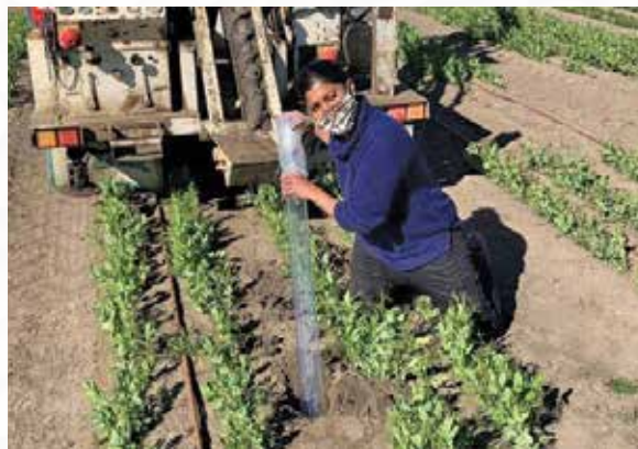
Dr Shiwangni Rao installing a rhizotron tube as part of her field research at the Agriculture Victoria Research Horsham SmartFarm
