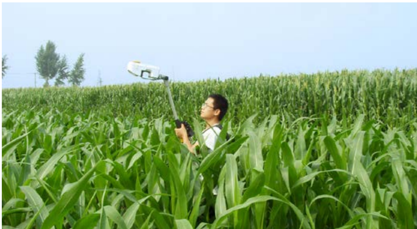
A student uses the GreenSeeker active canopy sensor to collect canopy reflectance data. The collected data will help determine the crop's nitrogen status.
