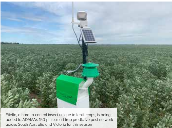
A smart insect trap installed in a faba bean crop as part of the ADAMA Trapview Predictive Pest Network
