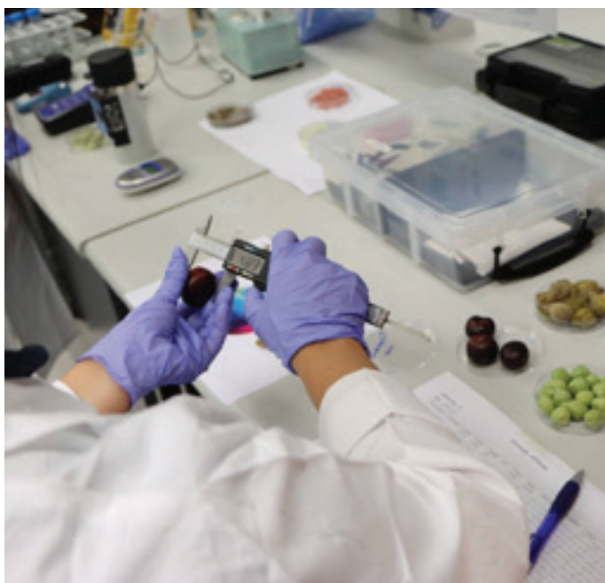
Image: Dr Anh Phan demonstrates use of callipers to measure fruit to seed ratio – equipment included in the chemistry toolkit, Coopers Plains Lab
