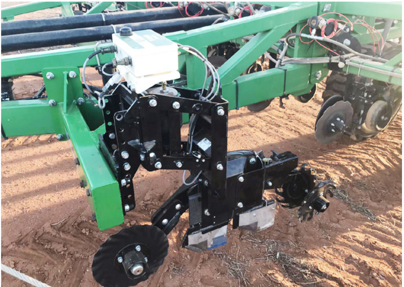
Photo caption 5: Pictured is a prototype of the iScan deep soil mapping module mounted on an Ausplow DBS seeding bar, which collects soil samples and data from thousands of sites in each paddock for generation of soil pH, nitrogen, organic carbon, electrical conductivity (EC), moisture and temperature maps. Paddock maps also are expected to be produced for other key soil elements as the technology further develops.
